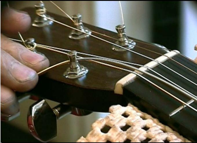
1 Position the machine-head capstan hole so that it is parallel with the nut. Thread the string through the hole and pull most of the slack out of the main body of the string, leaving about 3cm or 1".
