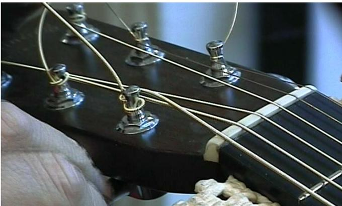
5 As the machine-head capstan is rotated, the string end should be well secured against the post, allowing the least amount of turns before the correct pitch is reached.
