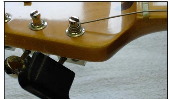
6. By the time the string is up to tension, there should be 3 wraps (minimum) on the post. This will ensure the string has greater grip because there is more surface area with the post.
