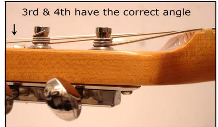
12. Once the Restring is completed with the correct angles, the guitar will stay in tune. All that remains is to 'Pre-tension the Strings' as explained in the following text.....
