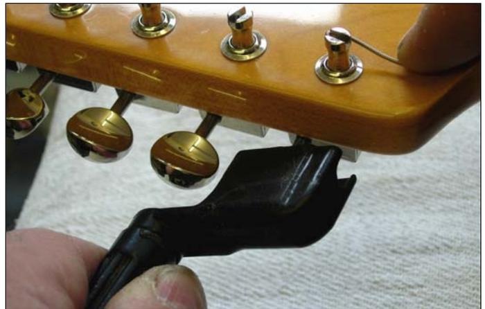
4. Press the string into the slot, bending it so it is horizontal (parallel with the headstock). Turn the tuning button anti-clockwise so the string starts to wind onto the capstan.
