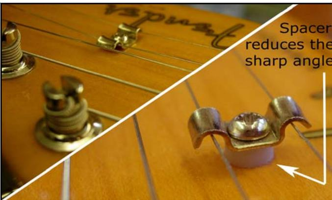
1 One modification is to fit a small spacer under the string tree to reduce the sharp angle off the nut. This should give enough down-pressure but still allow free movement of the string when using the tremolo (if fitted).
