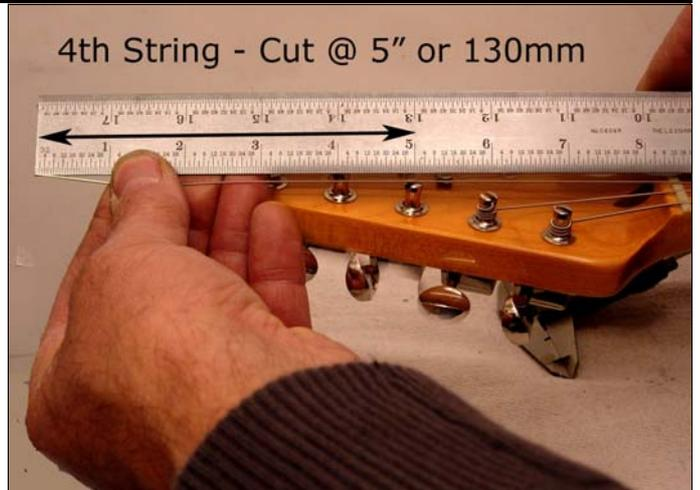
8. Measure & cut 5" or 130mm past the 4th post. This gives you enough winds so that it finishes at the bottom of the post and increases the angle of the string off the nut, giving greater down-pressure.
