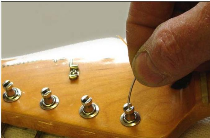
3. If the string was cut cleanly, the end should be easily pushed down the hole in the centre of the capstan until it won't go any further.
