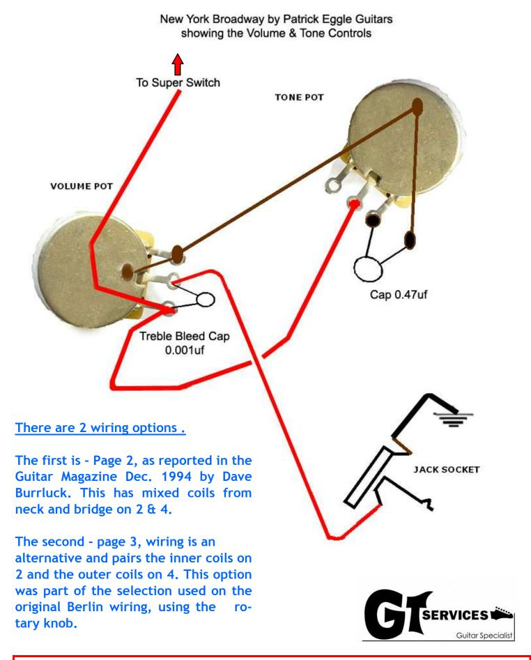
The New York Broadway uses a chrome covered mini humbucker, If this has been fitted incorrectly, please turn the pickup around 180° to get the wiring shown.
