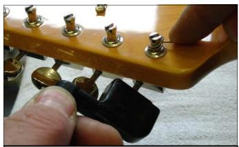
5 As the machine-head capstan is rotated, the string end should be well secured. The string wrap must go DOWN the post in order to give the right amount of down-pressure on the nut.
