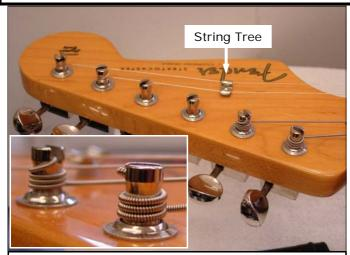
Once the 1st, 2nd, 5th & 6th strings are fitted a different method is used for the 3rd & 4th because there is no string tree to give enough downward pressure. Ignore the following if you do have 2 fitted.
