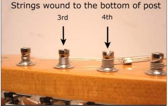
10. This is how it should look after the restring is complete. Note that the 2nd and 5th strings only have the necessary 3 turns to give good grip on the post..
