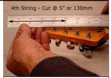
Measure & cut 5" or 130mm past the 4th post. This gives you enough winds so that it finishes at the bottom of the post and increases the angle of the string off the nut, giving greater down-pressure.
