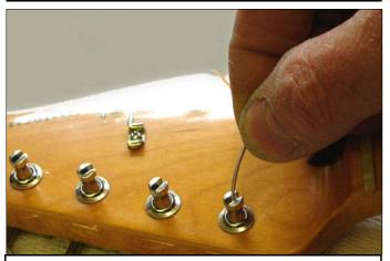
If the string was cut cleanly, the end should be easily pushed down the hole in the centre of the capstan until it won't go any further.
