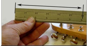
Finally, for the 3rd string, measure & cut in a similar way to how the 4th string was done but @ 6" or 150mm and wind the remaining string to the bottom of the post.
